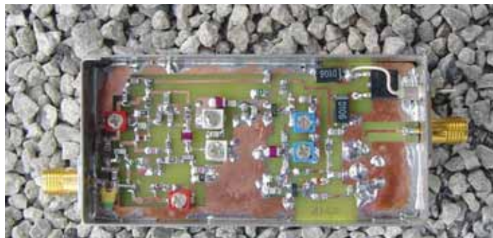
PHOTO 1: One of the prototype sources. This version uses different trimmer capacitors to those specified. The red trimmers shown are now replaced by black bodied 4 to 25pF trimmers.
