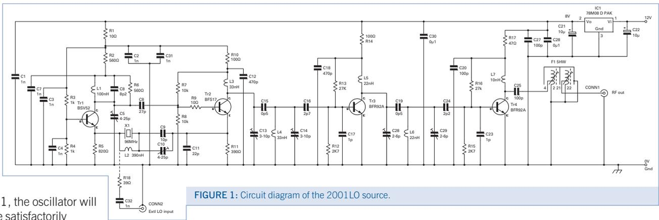
FIGURE 1: Circuit diagram of the 2001LO source.
